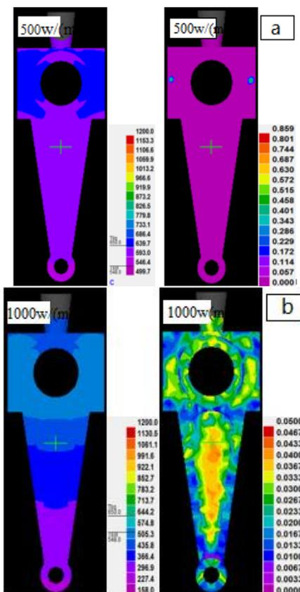
**Fig.4** The effect of coefficient of heat transfer on solidification time and state:
