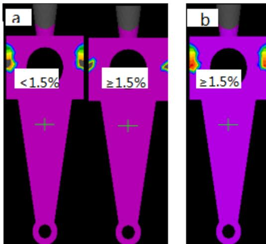
**Fig.6** Distribution of casting shrinkage porosity and cavity:
