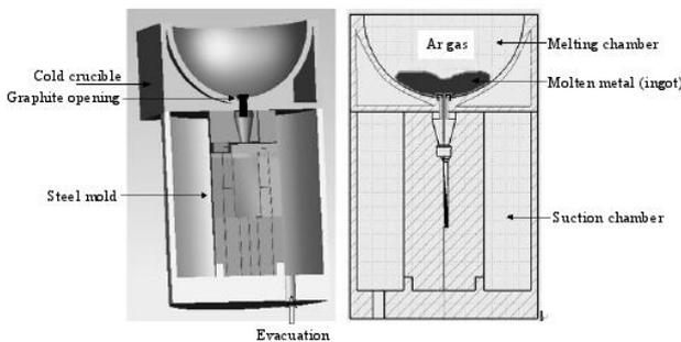
**Fig.1** Schematics of suction casting
